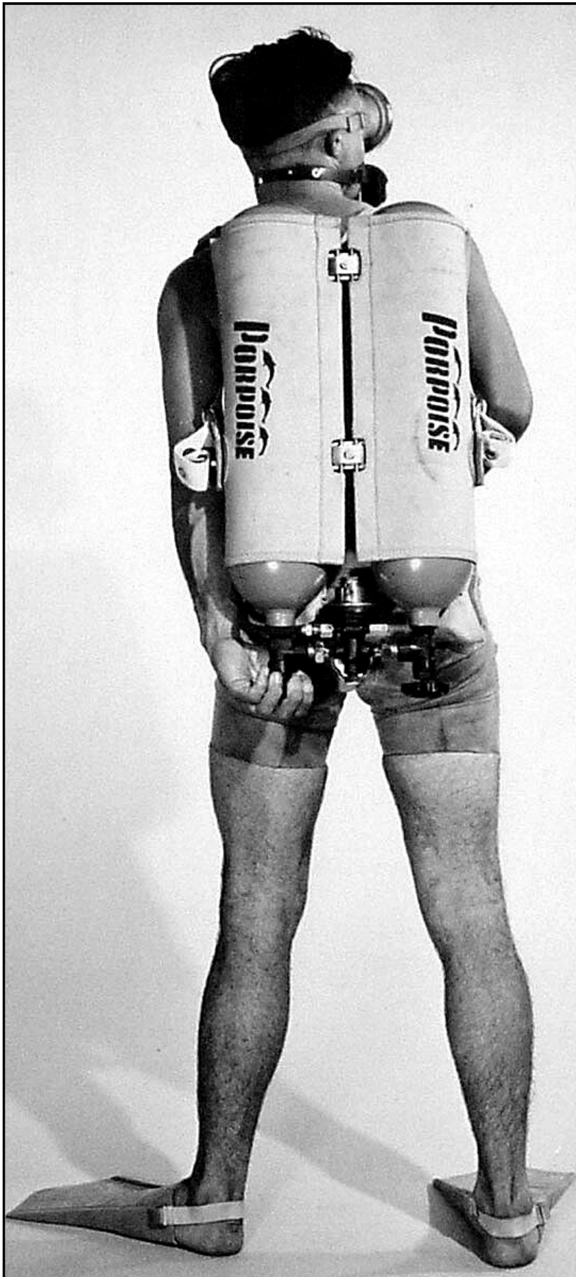
A rare image of the Porpoise CA2 twin cylinder configuration with buoyancy backpack
